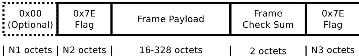
Figure 3.3. Amateur Bell 202/HDLC frame format
